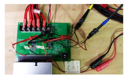
Figure 4: Sense Line, when provided, is used to measure the output voltages
