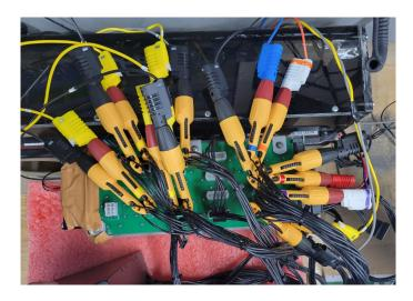
Figure 3: Insulated Piercing Probe to Measure the Output Voltage of Desktop Power Supply
