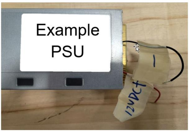
Figure 8 External Fan Power Labeled
